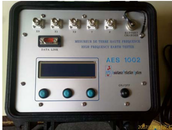
A typical High Frequency Earth Meter based on variable frequency injection: AES1002
